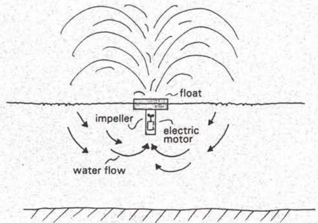
■ **Impeller-Aspirator** systems consist of an electric motor-driven impeller at the bottom of a hollow shaft extending at an angle down into the water. The assembly floats on the lake surface. The rapidly-turning impeller draws air down the shaft and propels water and air bubbles into the lake. Aeration takes place through air bubble/water contact and at the agitated lake surface.
